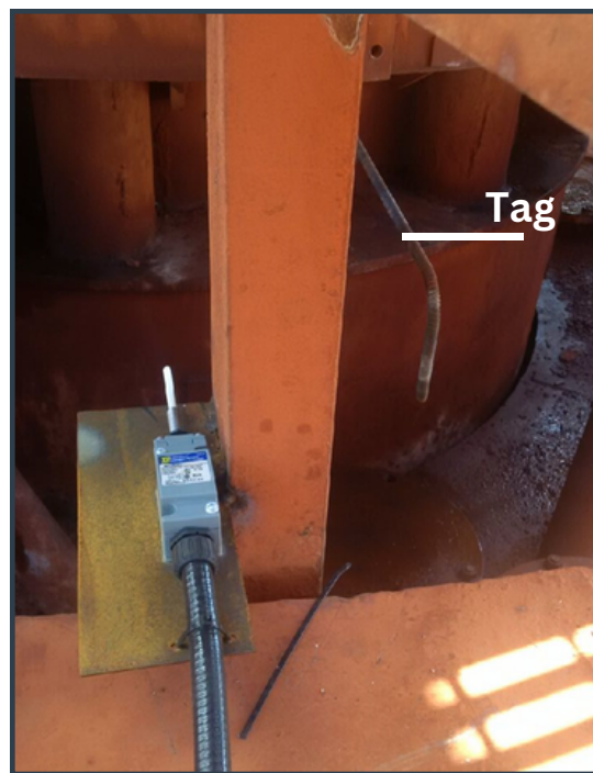
A Tag rotates on the Rake Drive, which triggers the Switch Arm.
