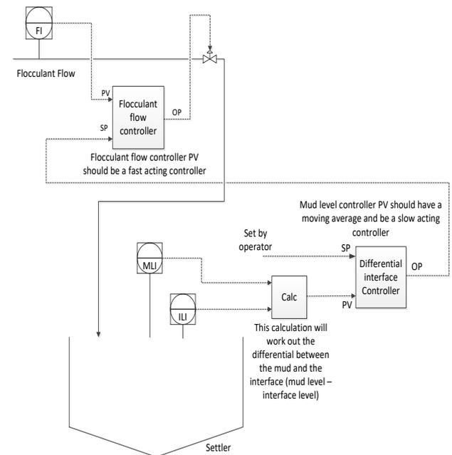
Figure 6. Interface control using the PLA SmartDiver
