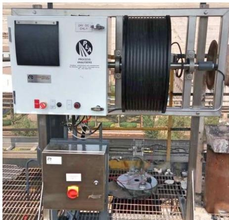
Figure 4. Retraction mechanism utilised by the SmartDiver
