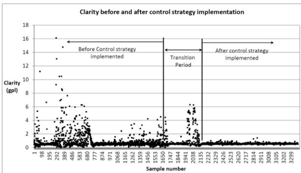
Figure 9. Chart showing clarity before and after implementation of feedback and feed-forward or model-predictive control
