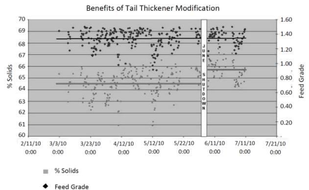
Figure 10 Change in thickener underflow density utilising a similar control strategy (Weidenbach and Lombardi, 2012)
