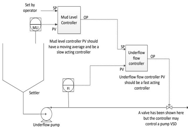
Figure 5. Mud level control utilising a PLA SmartDiver
