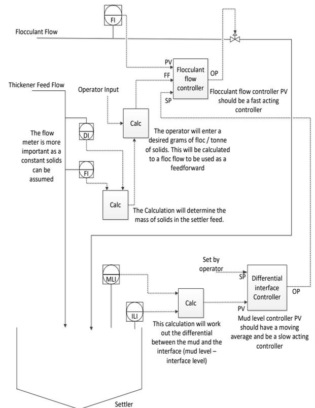
Figure 8 Interface level control with feed-forward utilising the PLA SmartDiver
