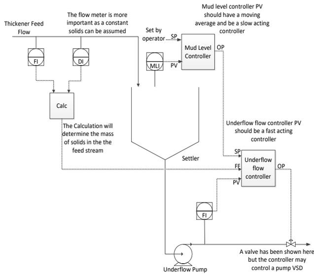
Figure 7. Mud level control with feed-forward using the PLA Smartdiver
